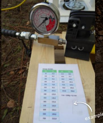
The step size is initially based on 2kN for horizontal. After performing the first test, it can be assessed to what extent this step size needs to be further refined.
