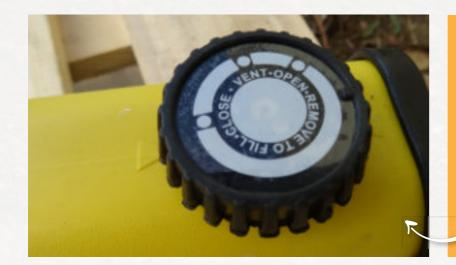
After the hand pump has been connected to the cylinder via the hydraulic hose, make sure that the black screw cap of the oil reservoir is turned from "Close" to "Vent". This must be set to ventilation, otherwise the pump will create a vacuum.
