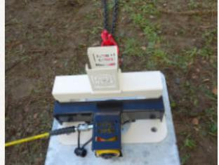
Mount the hydraulic cylinder in the adapter
