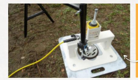
Mount the analogue displacement meter on the tripod and position the displacement meter exactly above the ground screwfoundation.
