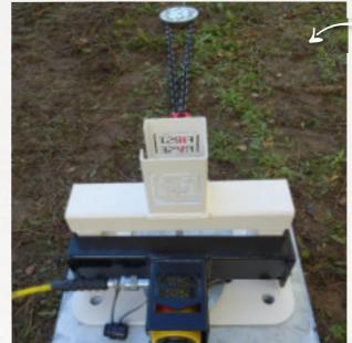
Mount the analogue displacement meter on the tripod and position the displacement meter exactly above the ground screw foundation in a horizontal direction.
