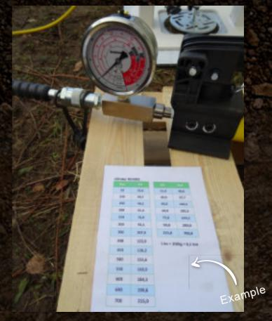
The step size is initially based on 15kNfor vertical. After performing the first test, it can be assessed to what extent this step size needs to be further refined.
