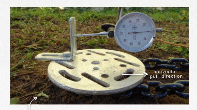
By mounting a bracket on the flange plate, a vertical support surface can be created for the analogue displacement meter.
