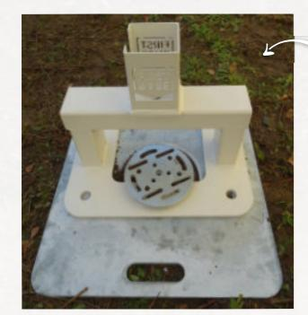
Place the TP-100 Horizontal Adapter against the side of the test frame, with the protruding head plates downwards.
